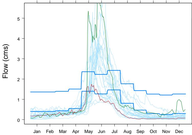
Figure 7. Spahomin Creek flows (08LG060). Light blue lines indicate daily flows, overlaid for the years 1972 through 1996. The green line indicates flows in the year 1995, a relatively wet year. The red line indicates flows in 1977, a relatively dry year. The dark blue lines indicate calculated minimum and maximum flow thresholds, based on the BC Instream Flow Guidelines.
