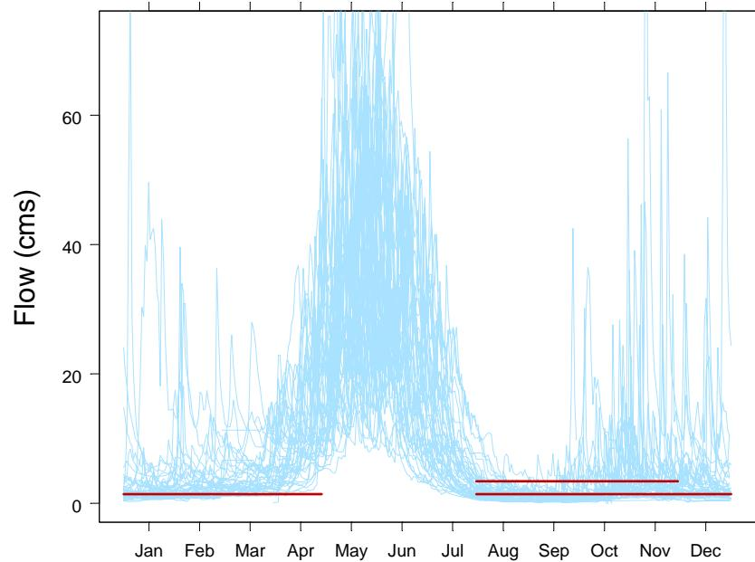
Figure 5. Coldwater River flows at Merritt (08LG010). The lower red line indicates 50 cfs ( $1.42 \text{ m}^3 \text{ sec}^{-1}$ ), the "Fisheries Resource Maintenance Flow" recommended by Kosakoski and Hamilton (1982). The upper red line for months of August through November indicates 120 cfs ( $3.4 \text{ m}^3 \text{ sec}^{-1}$ ), the optimum spawning flow as calculated by Kosakoski and Hamilton.
