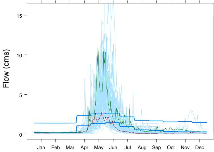
Figure 8. Pennask Creek flows (08LG016). Light blue lines indicate daily flows, overlaid for the years 1920 through 2003. The green line indicates flows in the year 1997, a relatively wet year. The red line indicates flows in 1977, a relatively dry year. The dark blue lines indicate calculated minimum and maximum flow thresholds, based on the BC Instream Flow Guidelines.
