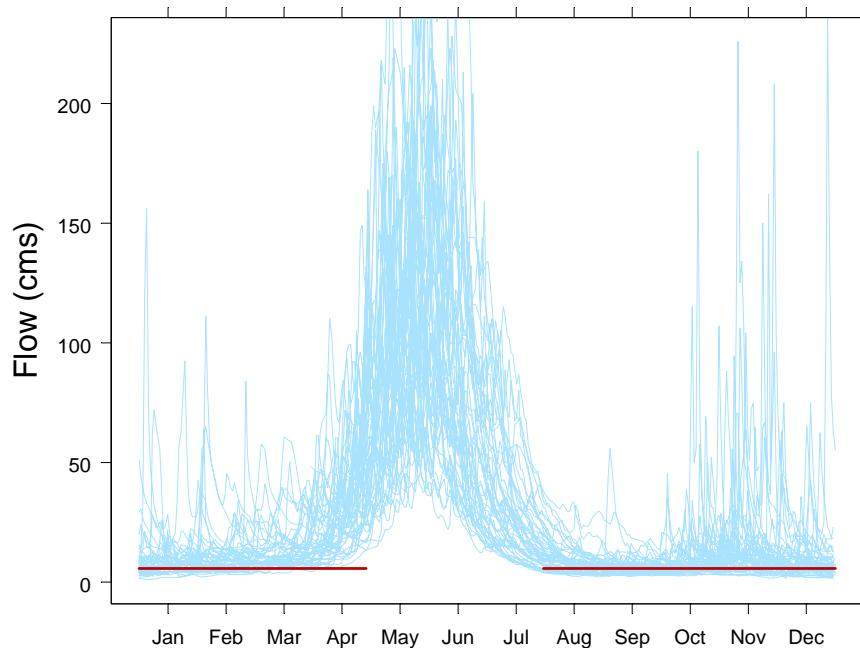
Figure 2. Nicola River flows at Spences Bridge (08LG006). The red line indicates 200 cfs ( $5.66 \text{ m}^3 \text{ sec}^{-1}$ ), the minimum flow recommended by Kosakoski and Hamilton (1982) for this portion of the river.
