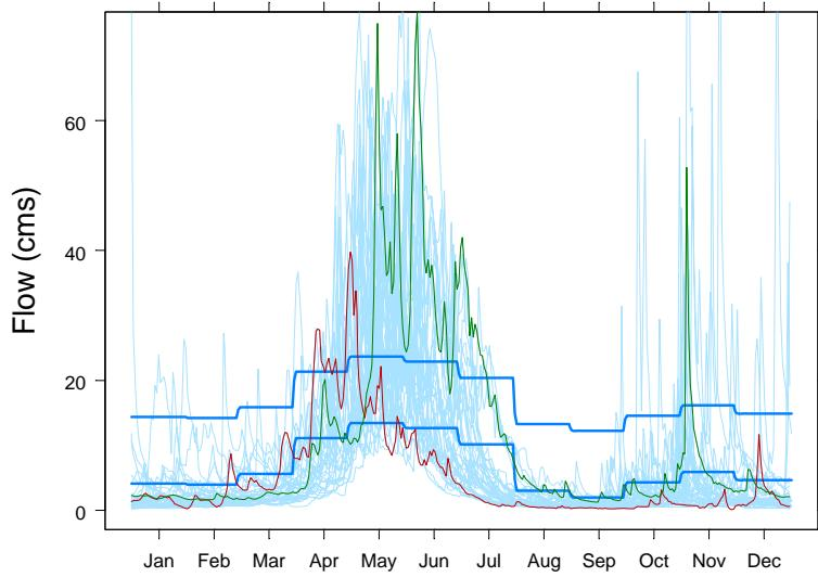
Figure 10. Coldwater River flows at Brookmere, based on naturalized data from MoE. Light blue lines indicate daily flows, overlaid for the years 1965 through 2003. The green line indicates flows in the year 1999, a relatively wet year. The red line indicates flows in 1994, a relatively dry year. The dark blue lines indicate calculated minimum and maximum flow thresholds, based on the BC Instream Flow Guidelines.
