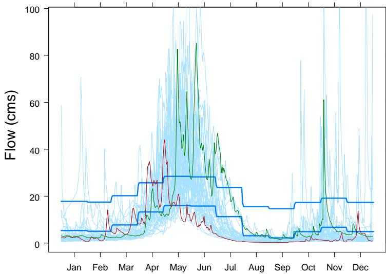
Figure 11. Coldwater River flows at Merritt, based on naturalized data from MoE. Light blue lines indicate daily flows, overlaid for the years 1965 through 2003. The green line indicates flows in the year 1999, a relatively wet year. The red line indicates flows in 1994, a relatively dry year. The dark blue lines indicate calculated minimum and maximum flow thresholds, based on the BC Instream Flow Guidelines.
