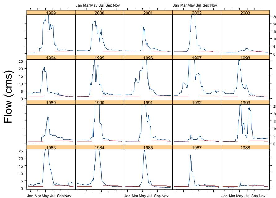
Figure 12. Outflow from Nicola Lake as recorded at 08LG65. The red line indicates 60 cfs ( $1.7 \text{ m}^3 \text{ sec}^{-1}$ ), the minimum flow recommended by Kosakoski and Hamilton (1982) for this portion of the river during the months of August through November, and 40 cfs ( $1.13 \text{ m}^3 \text{ sec}^{-1}$ ) for December through April.
