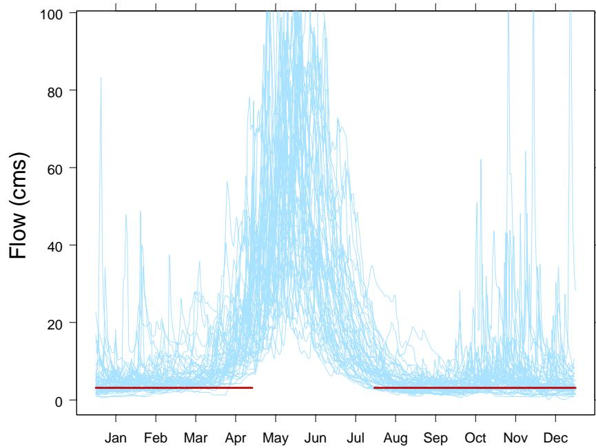
Figure 3. Nicola River flows at Merritt (08LG007). The red line indicates 110 cfs ( $3.11 \text{ m}^3 \text{ sec}^{-1}$ ), the minimum flow recommended by Kosakoski and Hamilton (1982) for this portion of the river.
