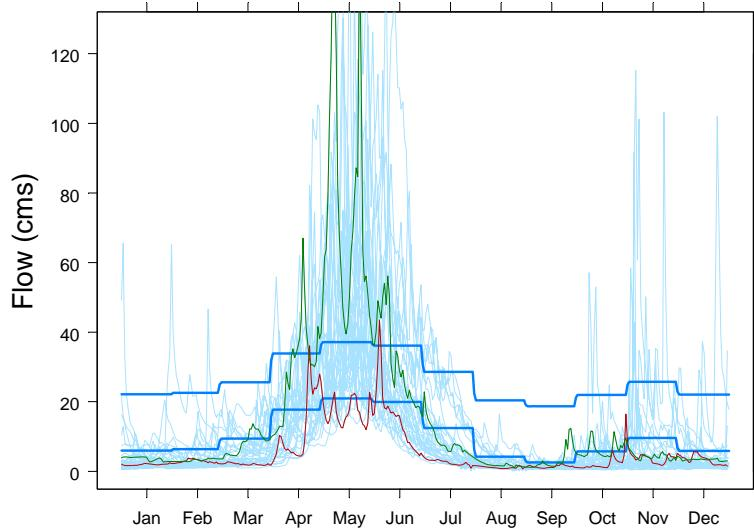
Figure 9. Spius Creek flows based on naturalized data from MoE. Light blue lines indicate daily flows, overlaid for the years 1970 through 2003. The green line indicates flows in the year 1997, a relatively wet year. The red line indicates flows in 1977, a relatively dry year. The dark blue lines indicate calculated minimum and maximum flow thresholds, based on the BC Instream Flow Guidelines.
